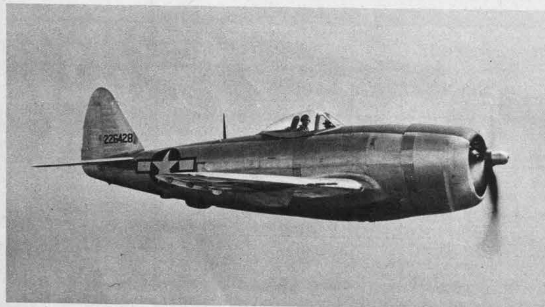
P-47D The Thunderbolt's chief external variation is the bubble canopy which appears to be replacing the faired type on most USAAF and RAF single-engine fighters. Wing rack for fuel tanks or bombs adds to P-47's versatility as escort plane, strafe and divebomber.
